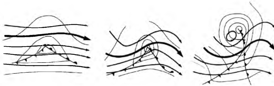
Figure 2.8 Schematic representation of the development of a cyclone wave. The heavier lines represent the flow at upper levels, with the heaviest line showing the most rapidly moving air. The frontal depression at the surface is denoted by the warm (semi-circles) and cold (triangles) fronts and by the lightest lines which represent the surface isobars (lines of constant atmospheric pressure). Adapted from McIlveen (1992) (see p. 32 Note 13).
