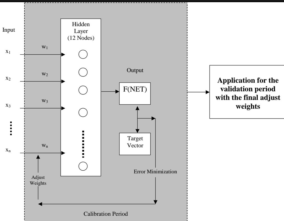
Figure3. The artificial neural network model used.
