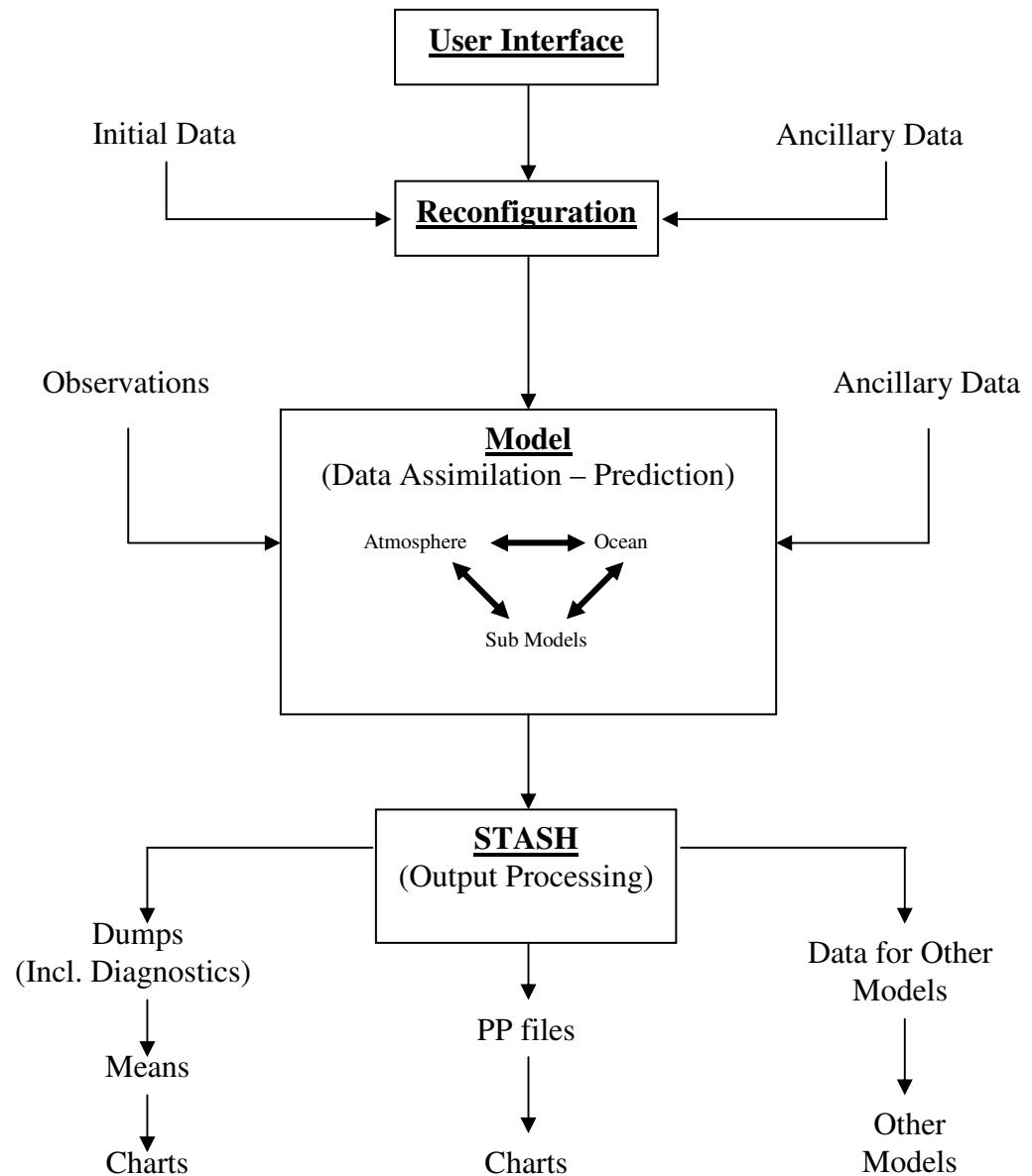
**Figure 6.4:** The Unified Model software system (after Cullen, 1993; Met. Office, 1996).
